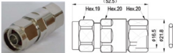
N Straight male Connector for 1/2" Flexible RF Cable
